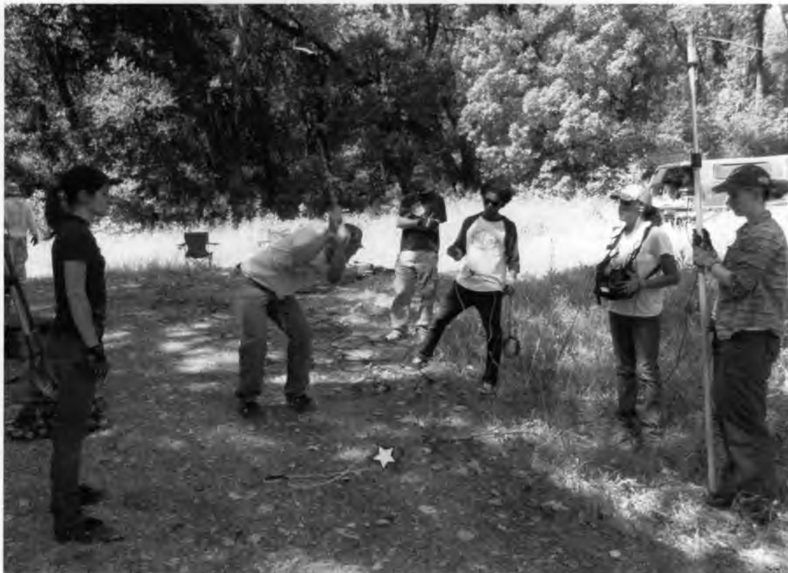
Figure 10: Photo showing method for P-wave generation. A hammer is used to trigger data recording when hit vertically on a steel plate (denoted by yellow star) placed every 1 m.
