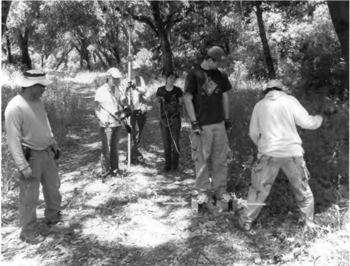
Figure 11: Photo showing method for S-wave generation. An aluminum box with cleats (to add shear to the surface) is placed every 1 m, while a hammer is used to trigger data collection. The block is struck on both ends multiple times (signified by yellow arrows) to force the block to move perpendicular relative to the seismic profile.
