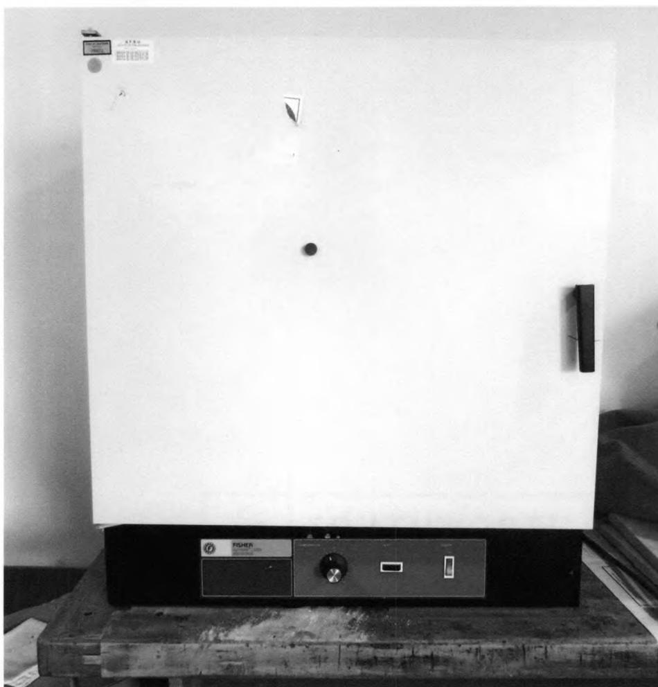
**Figure 14:** Drying oven used in porosity measurements. Oven is located in Hensil Hall room 112 at SFSU.
