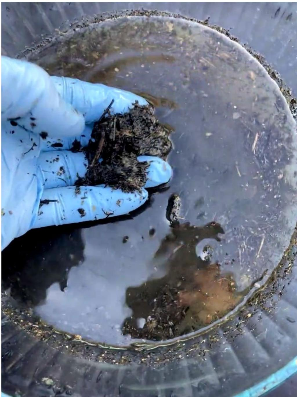
**Figure 8. Trace amounts of sand were collected in bedload transport sampling during the pulse flows of 1,500 cfs in February 2022. The mesh size of the TR-2 sampler is 0.5 mm.**
