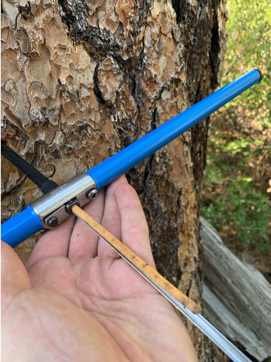
Figure 5 Hagloff increment borer and Pinus ponderosa core.
