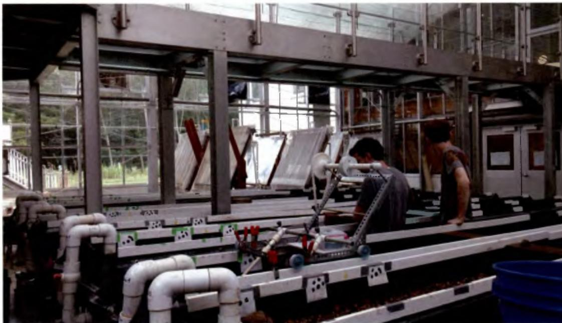
Figure 6) The Stroud Water Research Center's indoor river laboratory in Avondale, Pennsylvania. The flumes provided caddisflies with habitat and water was sourced from nearby White Clay Creek, which also organic particulates which was a food source for the insects. The lab contains 10 flumes, 3.3 m long, 0.4 m wide and 0.3 m deep.
