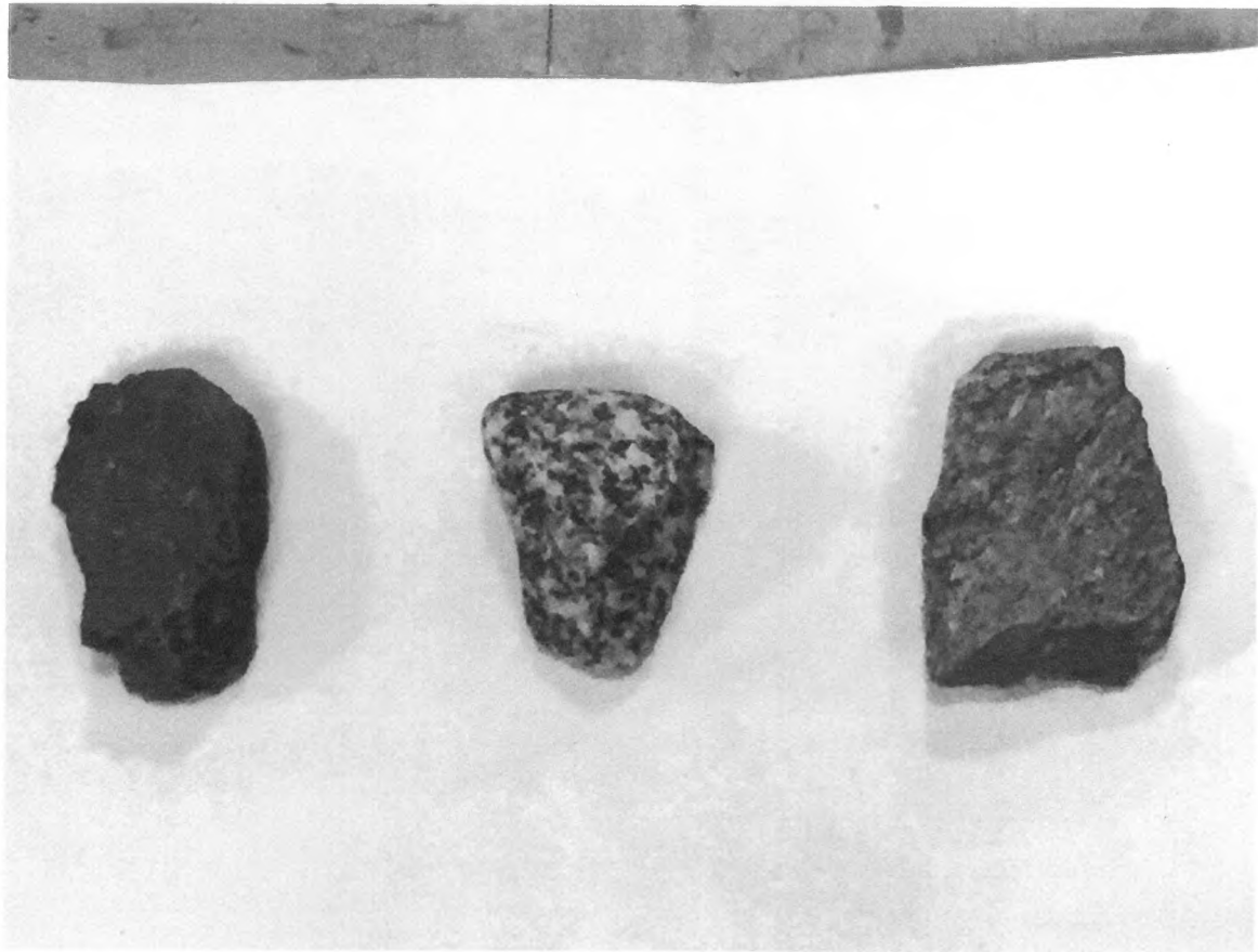
Figure 3: Rock types used in the free-fall single-particle and rotating drum experiments. From left to right: basalt, granodiorite, and serpentinite.
