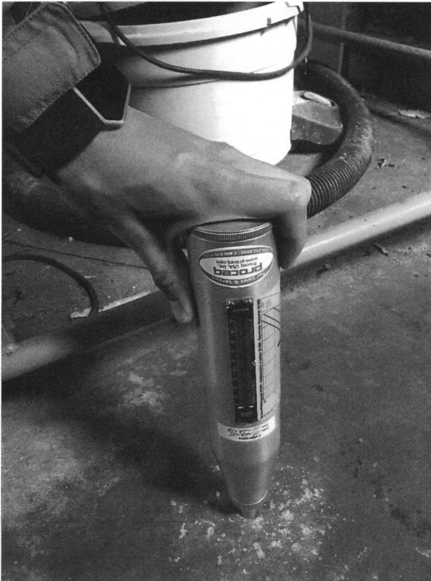
Figure 5: Measuring the compressive strength of one of the drop locations with the Schmidt hammer.
