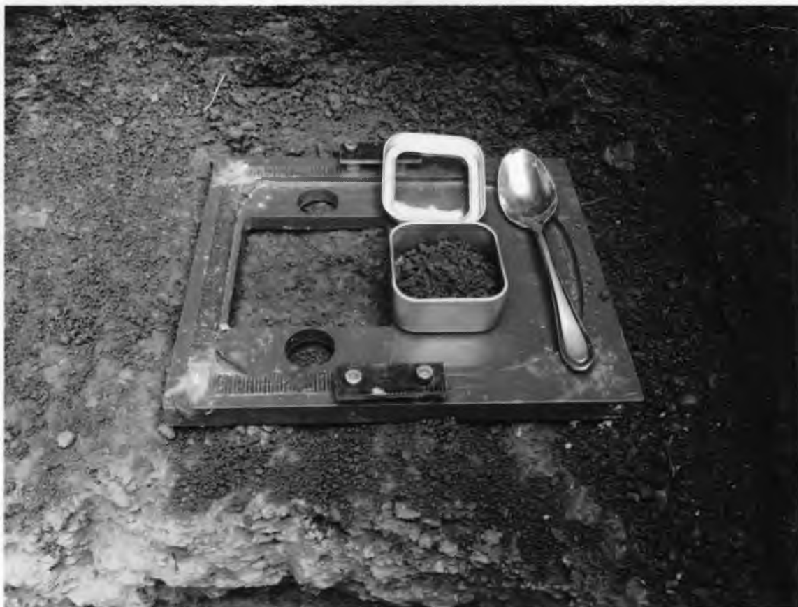
Figure 7: MILT platform and soil sample in heat-resistant tin. Spikes on the bottom of the platform anchor it to the soil to maintain MILT's position between scans. Window in platform allows the MILT's lasers to image soil surface.
