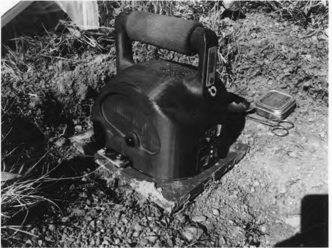
Figure 4: NASA's Mold Impression Laser Tool (MILT) with USGS template, a portable 3D scanner on custom platform in the field during bulk density measurement.
