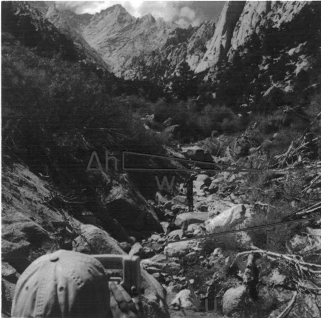
Figure 13: Field survey of debris flow track at Inyo Creek, CA, with the terms in the super-elevation calculation annotated.
