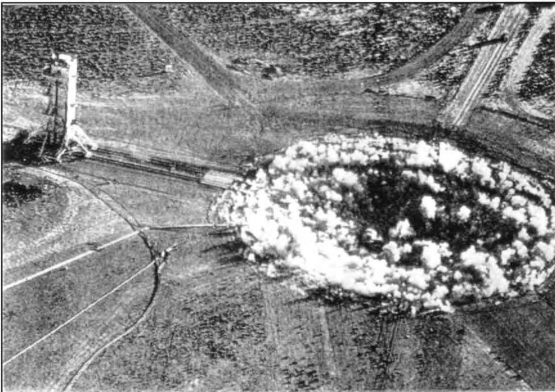
The ten story tall instrumentation tower on the left was winched away from the drillhole before subsidence. LLNL photo.
