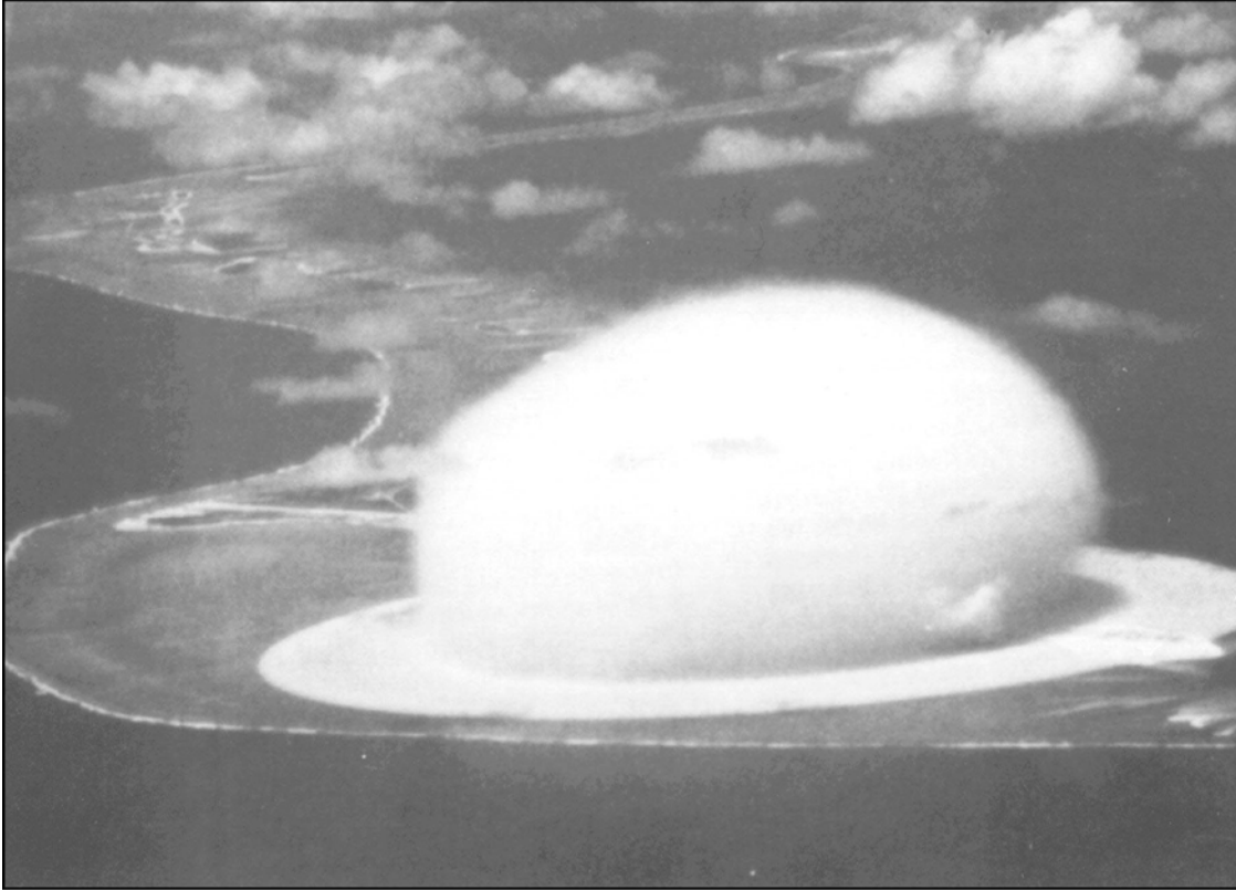
Thirteen kiloton SEMINOLE shot, June 1956. SEMINOLE was detonated in a tank of water to simulate a subsurface blast. AEC photo.
