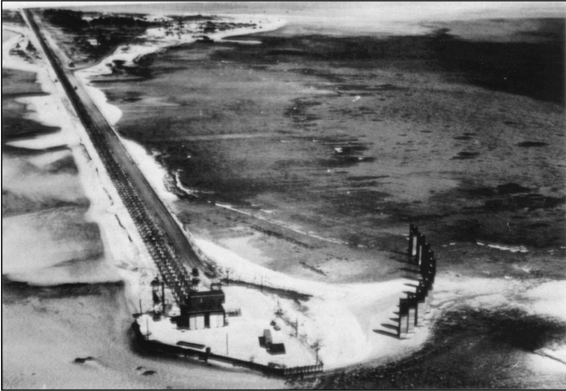
CASTLE/BRAVO shot area. Array of mirrors on right reflect early explosion effects to cameras stationed miles away. AEC photo.
