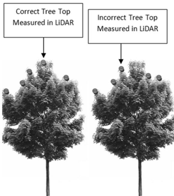
**Figure 11. Example of how LiDAR points can miss the top of tree and result in an incorrect tree height measurement in the LiDAR**
