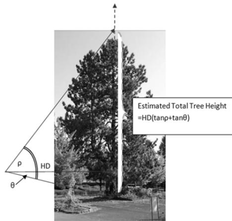
**Figure 3. Conventional field method of measuring tree heights in the field using trigonometric principles**
