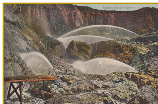
Figure 6: Hydraulic mining was used to access the gold deposits in the Sierra Nevada during the Gold Rush. Photo source: Cali49, 2016
