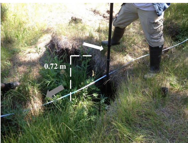
Fig. 12. Surveying a sod bridge in Rowland Creek. The white arrow indicates the top of the bridge; the gray arrow indicates flow direction.
