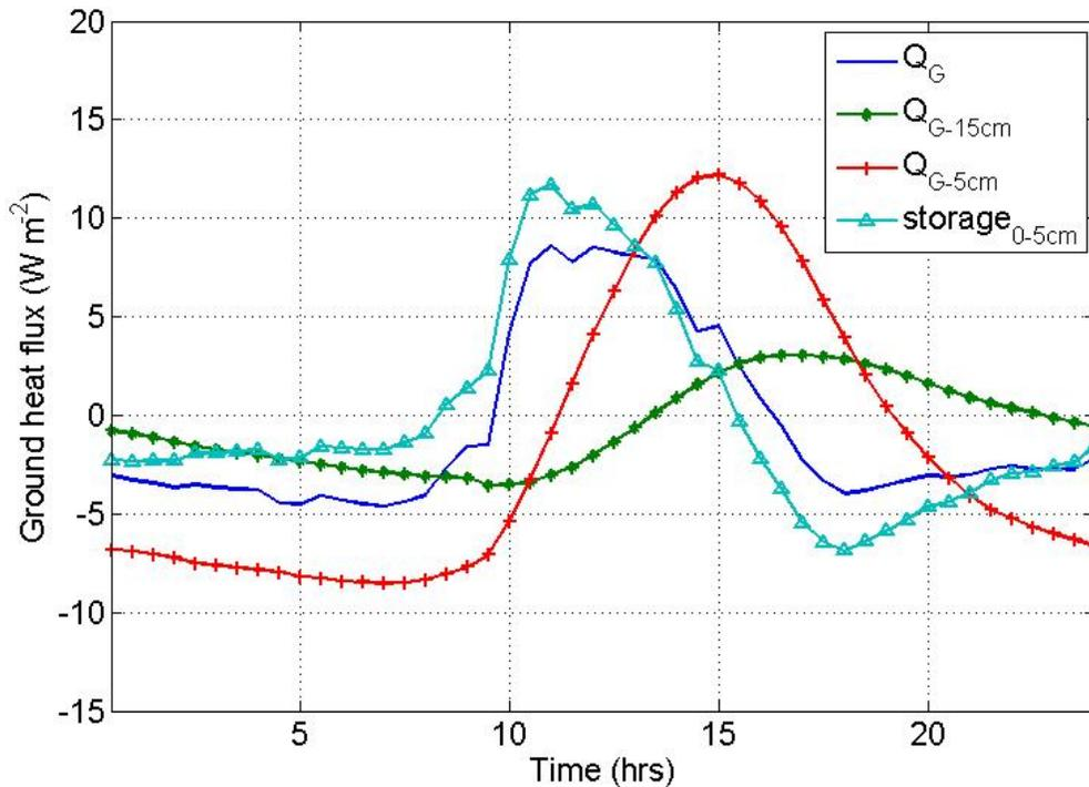
Figure 12. Partitioned diurnal ensemble ground heat flux terms for October – December 2014, where  $Q_G$  is the total ground heat flux,  $Q_{G-15cm}$  is the ground heat flux measured at -15 cm,  $Q_{G-5cm}$  is the ground heat flux at -5cm, and  $storage_{0-5cm}$  is the change in heat storage between -1 and -5 cm. Measured on the living roof of the California Academy of sciences, San Francisco, Ca.
