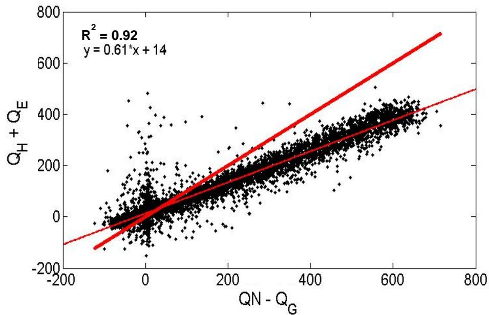
Figure 16. Energy balance closure (April 2014 – March 2015) on the living roof of the California Academy of Sciences in San Francisco, CA, where the thick red line is the 1:1 line and the thin red line is the linear regression trend
