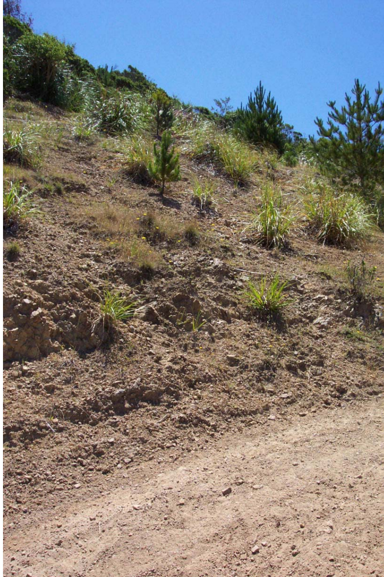
Figure 51: Rilling upslope of trail on terraced hillslope contributing to the sediment delivered to the drainage ditch in Figure 50 (Point 9 on Figure 47).
