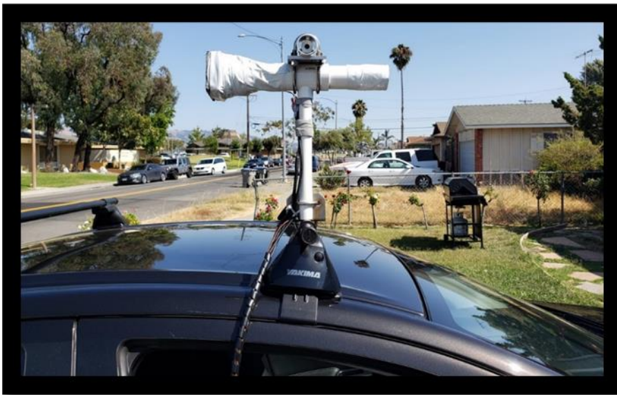
Figure 5: Vehicle with Mounted PVC pipe containing the type E thermocouple, HMP60 thermistor hygistor, Apogee infrared radiometer, and 12-volt fan.
