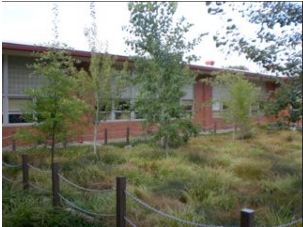
Figure 11: Rain garden catches runoff from roof via disconnected downspouts in Portland, OR. Photo by Alicia Omlid.
