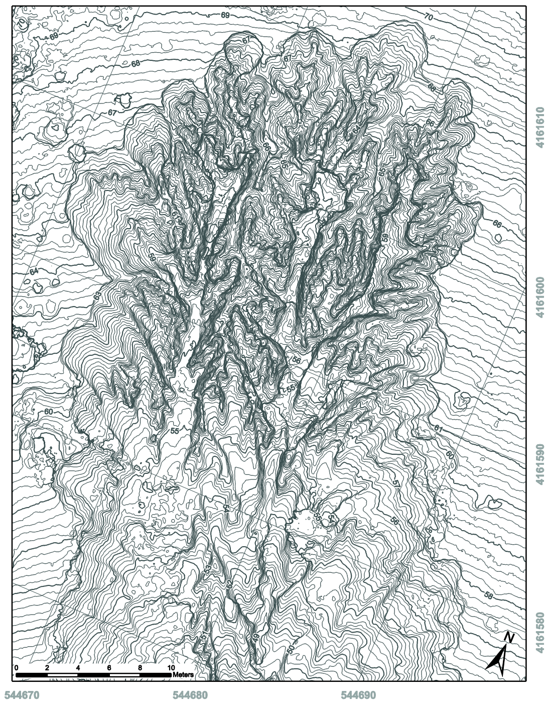
Figure 27. Digital Surface Model of 20m (33m average altitude AGL) Model derived from structure-from-motion methods employing Agisoft Photoscan. Contour interval: 0.2m. Index contours: 1m.
